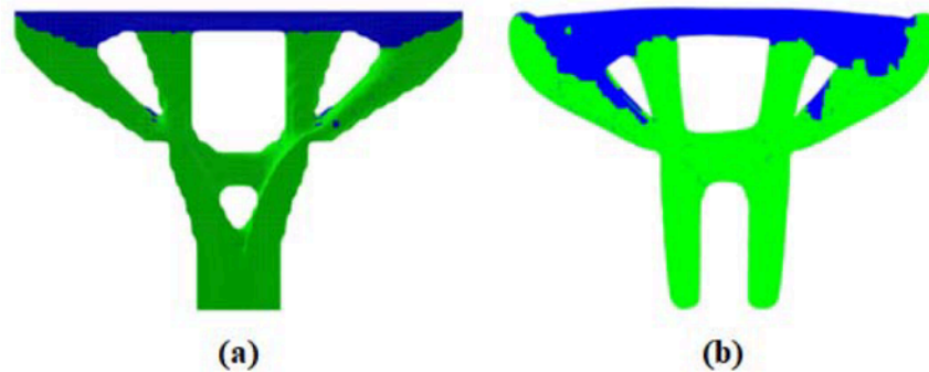
Fig. 17: Bridge Pier: Strut-and-tie models (a) SESO and (b) VFLSM
