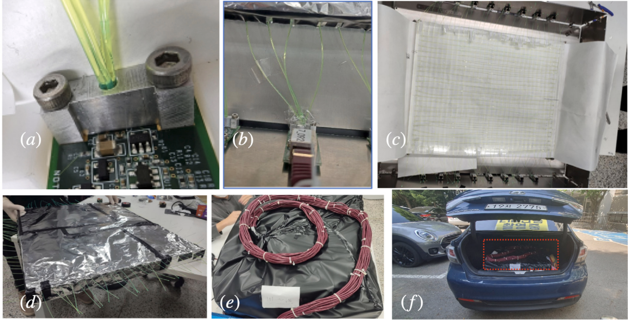
Fig. 3. Photos of the HAWL detector assembly. A front-end board connected with four fiber ends are shown in (a) and (b). The layout of the fibers with Tyvek sheets and additional aluminum foil covers are visible in (c) and (d), respectively. The completed HAWL detector is seen in (e) and it is set in place in the trunk of a sedan indicated by a red-dotted line (f) with the DAQ system in a back seat.
