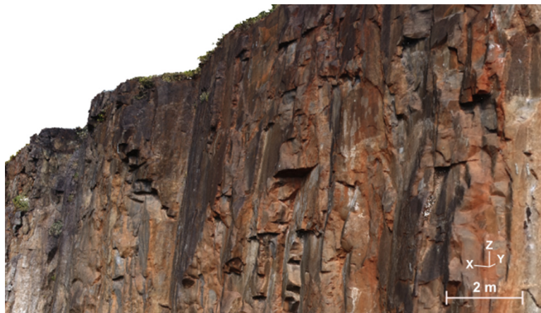
Fig. 7. Detail of the reconstructed dense cloud. Note that persistent horizontal and vertical planes were correctly reconstructed.
