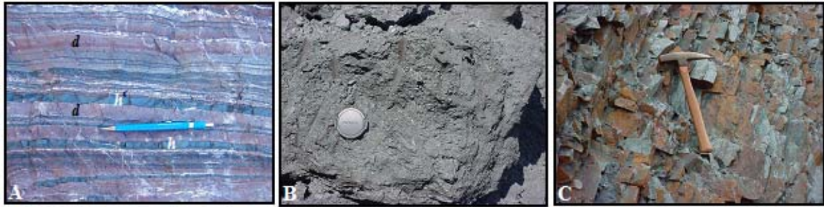
Figure 1 - Photographs of the protore and high-grade ores in the Águas Claras mine. A Hand specimen of dolomitic itabirite (protore) showing dolomite-rich (d) and hematite-rich (h) mesobands. B Soft Ore. C Outcrop of hard ore.
