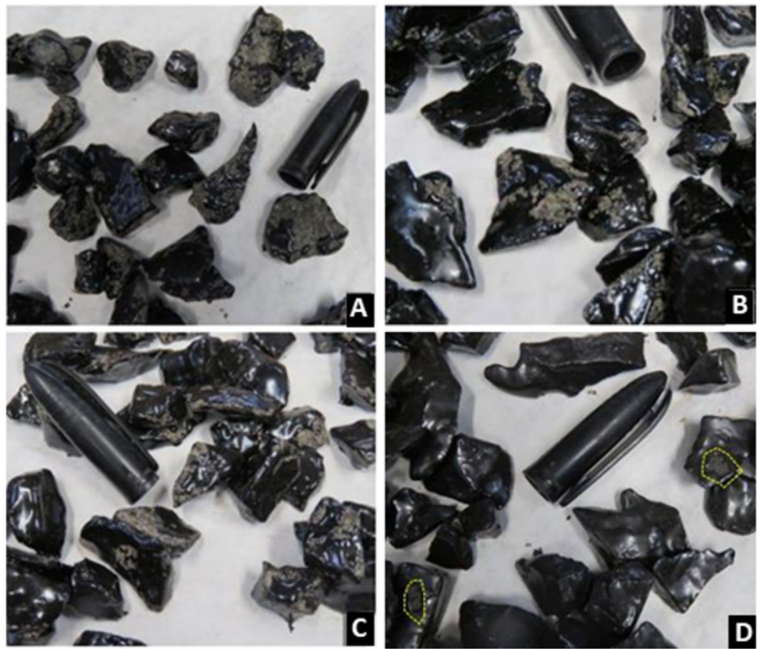
Fig. 11. Visual details of the aggregates in the CBB tests. Note the intense detachment of particles in (A) DIA diabase, (B) MON_M monzodiorite, and (C) MON_{MC} monzodiorite. In (D) More localized and less pronounced detachments of the asphalt cement in the APH basalt (details in dashed yellow).
