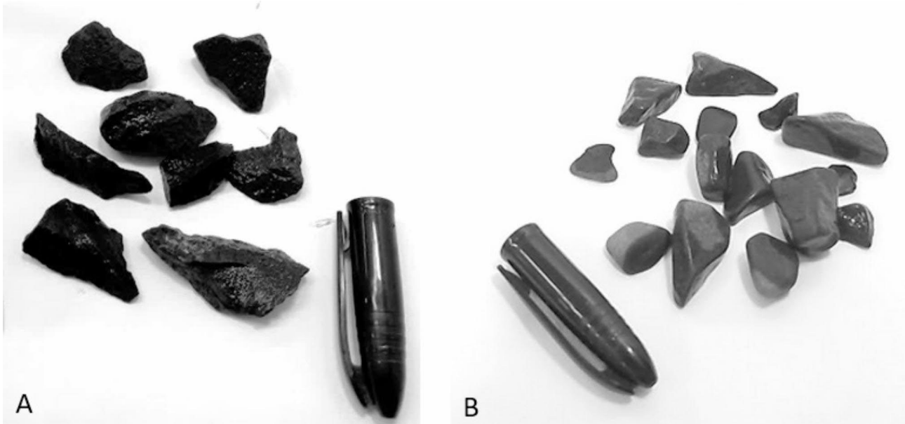
Fig. 8. APH basalt samples (Grade A) in MD tests: (A) Natural appearance of the fragments with rough surfaces before the tests; (B) Smooth surface appearance of the aggregates after being worn in the tests.
