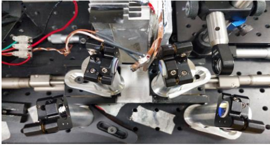
Figure 3: Photograph of the laser cavity, with the crystal in the center, coupled to an air cooling system.
