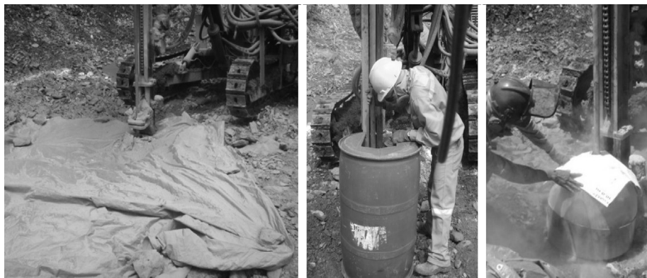
Figure 3 Blast hole sampling with three alternative approaches: canvas, drum and new sectorial sampler
