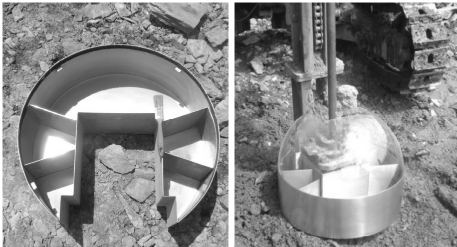
Figure 2 New modified sectorial sampler fitted to the PWH drill (right) and detail of the buckets/frame (left)
