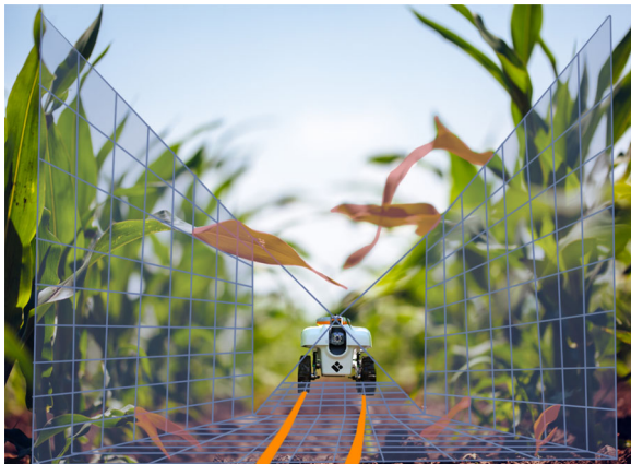
Fig. 1 Representation of our solution that autonomously navigates in farm row crops. By using perception through LiDAR and planning trajectories, our system can provide safe navigation in agricultural scenarios
